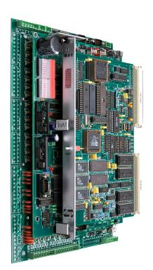
Incorporating analog and digital I/O capability, the Callisto™ Elara III remote provides a compact, cost-effective solution for complex SCADA applications
